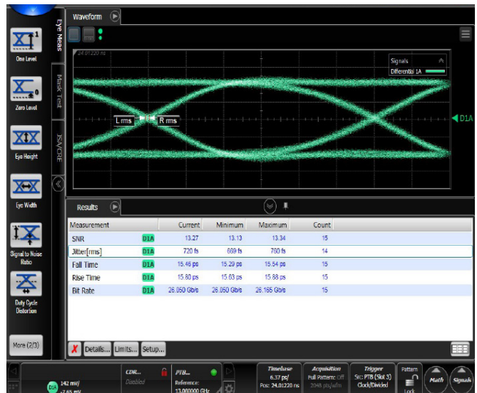
Example of 26 Gbps PRBS data signal generated using the low noise internal clock synthesizer.
