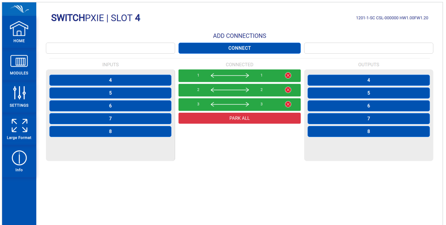
SwitchPXIe-1201 8x8 switch connection control in cohesionUI
