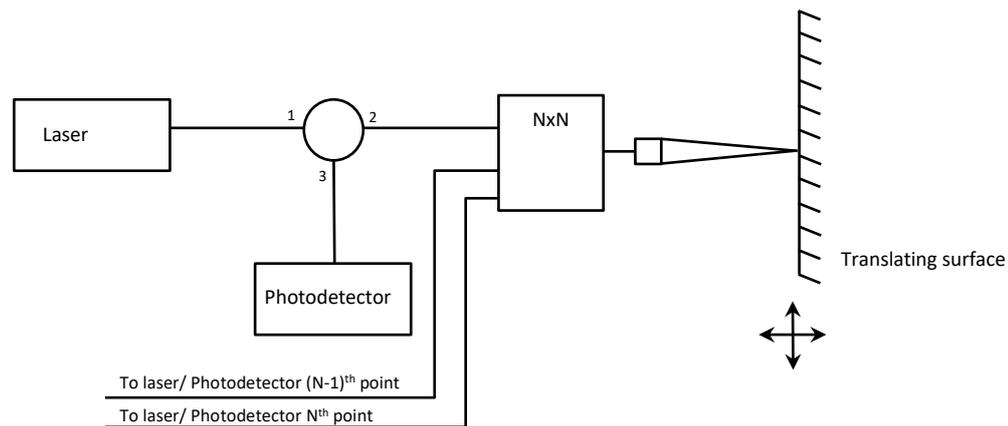
**Figure 5:** Leapfrogged Photon Doppler velocimetry
