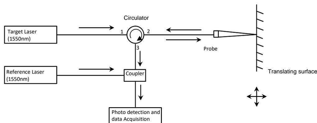
**FIGURE 1:** Simplified diagram of fibre-coupled PDV
